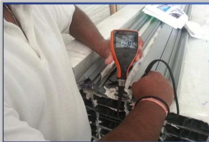
Verifying the thickness of coating
