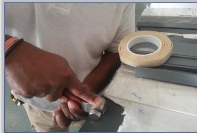
Scratch test to verify the coating adhesion
